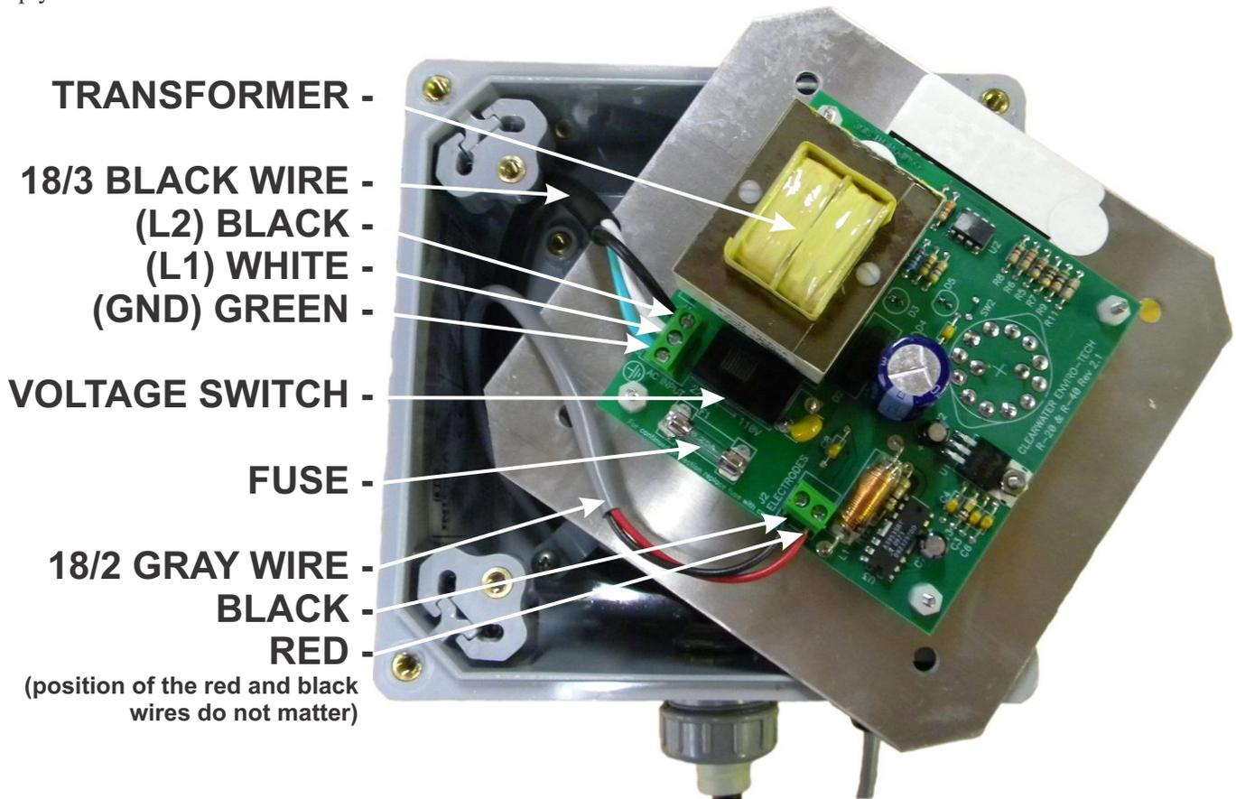
a.) The thick black power cord has three wires coming out of it - black, white and green. A green terminal with three screws (next to AC Input-printed on circuit board) houses these three wires. The far left terminal, **L2** should have a black wire going to it. The middle terminal, **L1** should have a white wire coming from it. The right terminal, **GND** should have a green wire coming from it (ground).
