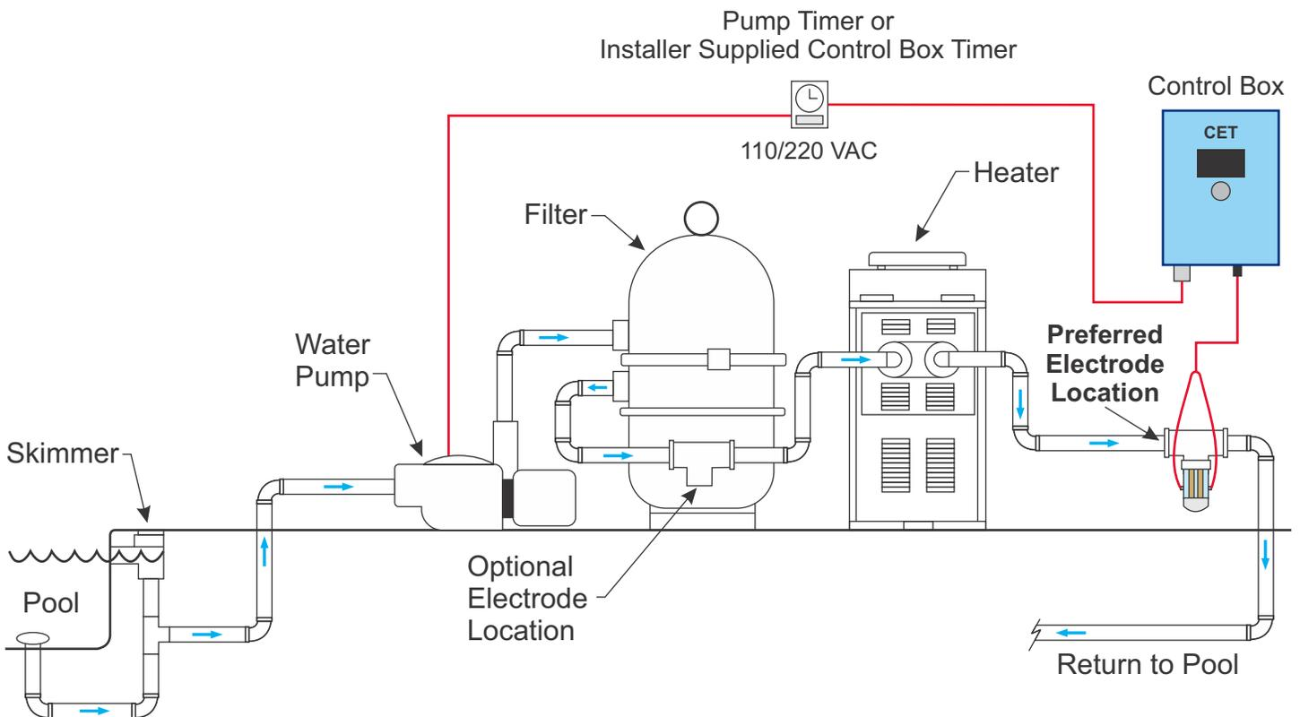
The **MineralPURE R-40** should be installed at the pool's pump and filter area. The preferable location to mount the electrode chamber(s) is after the pool's pump and filter, but it can be installed before the pool's pump and filter if needed. The electrode chamber(s) will need to be within 10 feet of the control box for an electrical connection. The control box will need to be within 7 feet of an electrical source.
