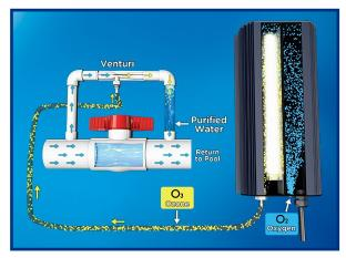
The **OzoneMAX** unit includes a side stream venturi manifold that injects the ozone into the water. As ambient air enters the ozone generator, the venturi creates a suction-effect to pull air past the UV bulb, creating  $O_3$  – ozone. The ozone is then safely injected into the water flow.
