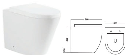
SRTWC6005 Washdown Flushing Technology Dimension : L560xW365xH400mm P-Trap : Horizontal Outlet 180mm *PP Material Seat Cover
