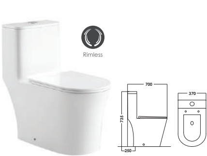
SRTWC8152-RL Washdown With Rimless Flushing Technology Dimension : L700xW370xH735mm S-Trap : Bottom Outlet 250mm P-Trap : Horizontal Outlet 180mm *PP Material Seat Cover
