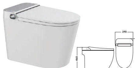
SRTWC189 Ceramic Intelligent Water Closet Siphonic Flushing Technology Dimension : L670xW380xH460mm S-Trap: Bottom Outlet 300mm
