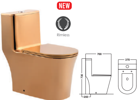
SRTWC8152-RL-RG Washdown With Rimless Flushing Technology Dimension : L700xW370xH735mm S-Trap : Bottom Outlet 250mm P-Trap : Horizontal Outlet 180mm *PP Material Seat Cover
