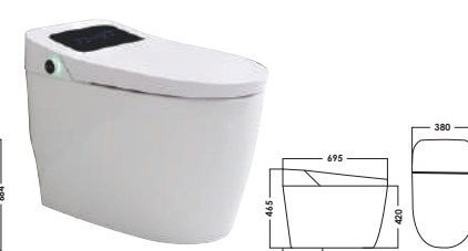
SRTWC018AF Siphonic Flushing Technology Dimension : L695xW380xH465mm Flush Volume < 4.0L (In dual flush mode) Water Efficiency : Grade 1
