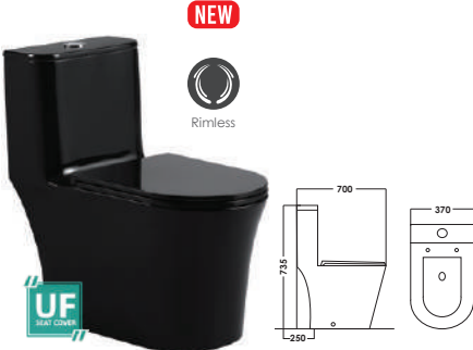
SRTWC8152-RL-BL Washdown With Rimless Flushing Technology Dimension : L700xW370xH735mm S-Trap : Bottom Outlet 250mm P-Trap : Horizontal Outlet 180mm *UF Seat Cover
