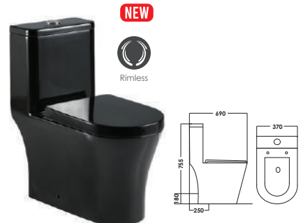
SRTWC8318-RL-BL Washdown With Rimless Flushing Technology Dimension : L690xW370xH735mm S-Trap : Bottom Outlet 250mm P-Trap : Horizontal Outlet 180mm *PP Material Seat Cover
