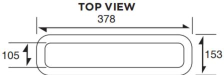
Dimension in mm Tolerance: ±0.03
