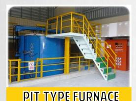
DESIGNED WITH CIRCULAR CONSTRUCTION. WITH INSULATED COVER WHICH IS HYDRAULICALLY LIFTED FOR CHARGING OR **REMOVING THE PRODUCTS INTO AND FROM** THE FURNACE. THE PRODUCTS CAN BE LOADED INTO THE PIT FURNACE WITH CRANE **OR SUITABLE LOADING MACHINE.**
