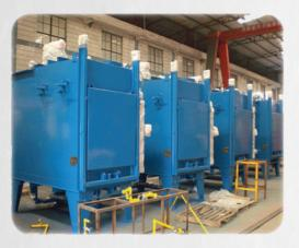
FOR APPLICATION OF RELIEVE THE INTERNAL STRESSES AND REDUCE BRITTLENESS OF METAL PARTS AFTER HARDENING.
