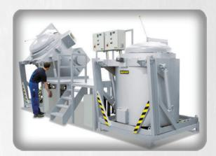
WITH HIGH MELTING OUTPUT, MOSTLY USED FOR MELTING COPPER ALLOYS, ALUMINIUM ALLOYS, ZINC ALLOYS AND ETC. IN PRODUCTION.
