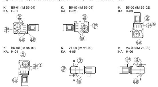
Figure 10-18 Type of construction options for KZ, KF, KM, KAD, KAZ, KAF, KAM, KADS, KAZS, KAFS, KADT, KAZT, KAFT sizes 38 - 188
