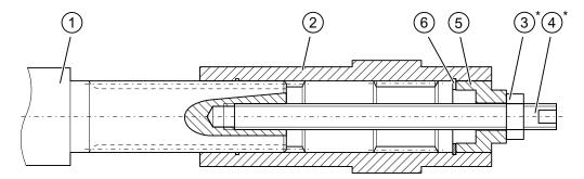
Figure 4-7 Installing the hollow shaft with splines
