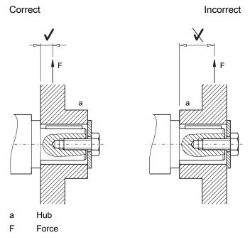
Figure 4-4 Mounting arrangement for minimum stress on shafts and bearings
