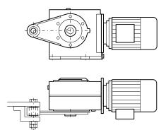
Figure 4-14 Mounting suggestion for torque arm on flange
