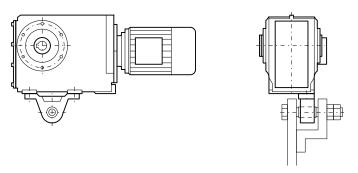
Figure 4-13 Mounting suggestion for torque arm on foot
