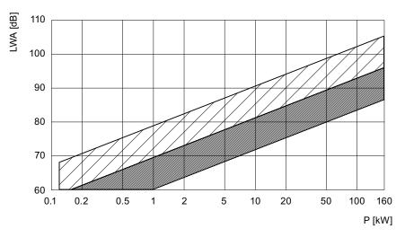
Figure 10-3 Sound energy level MOTOX geared motors
