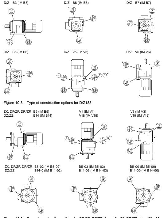
Figure 10-9 Type of construction options for DF/ZF, DZ/ZZ sizes 18 - 88, DR/ZR sizes 68 - 88
