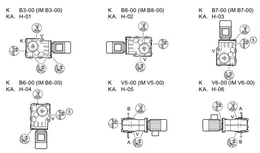
Figure 10-17 Type of construction options for K, KA, KAS, KAT sizes 38 - 188
