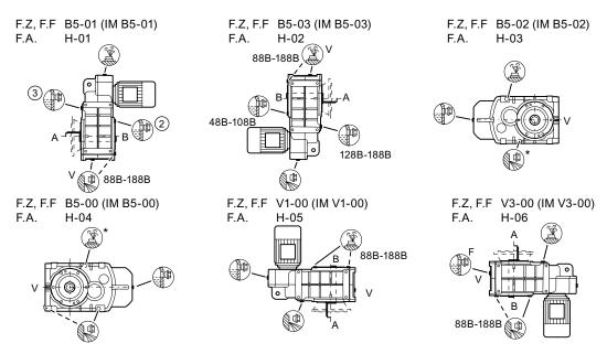
Figure 10-12 Type of construction options for F.28, F. sizes 38B - 188B
