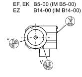
Figure 10-5 Type of construction options for E. sizes 38 - 148
