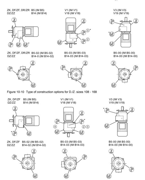
Figure 10-11 Type of construction options for D./Z.188
