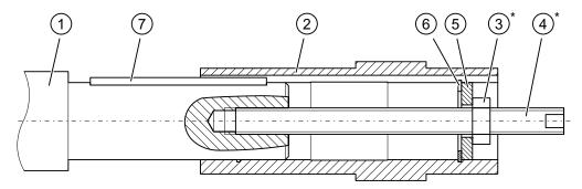
Figure 4-6 Installing the hollow shaft with parallel key
