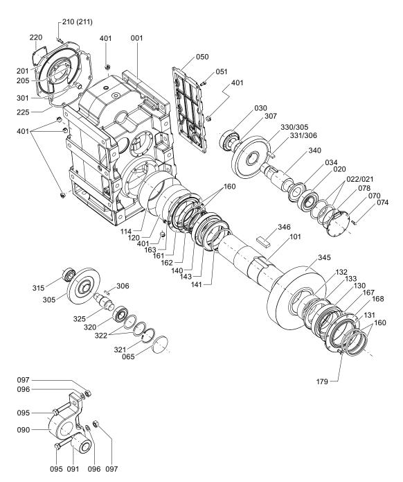
Figure 11-5 Parallel shaft gearbox size 208
