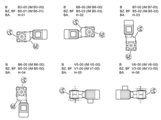
Figure 10-14 Type of construction options for B. sizes 28 - 38 without additional screw plug
