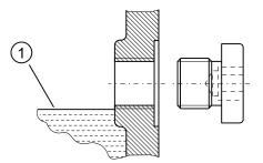
Figure 8-1 Oil level in the gearbox housing
