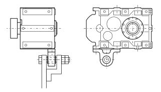
Figure 4-12 Mounting suggestion for torque arms on F.208
