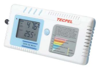
The ZG106 is a new and low-cost carbon dioxide monitor implementing IR-SoC technology. Its many features include a data logger that can record up to 24 hours of data, a CO2 level alarm, and an extreme level indicator.
