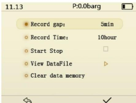
Display data: By means of the menu item "View DataFile", you can open and display the CSV data file via the device.
