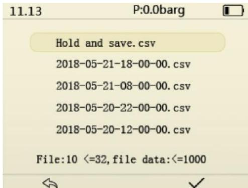
To view the saved data, press the right or left key. To view the next or previous data, press the up/down arrow keys to scroll through the data in steps of ten.
