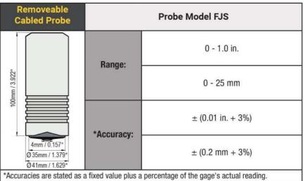
*FJS* - Removable FJS probe for measuring thick protective coatings on ferrous metal substrates. Ideal for thick epoxy, rubber, intumescent fireproofing and more.
