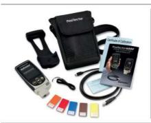
Comes complete with PosiTector gage body, FJS probe, precision plastic shim(s), protective rubber holster, wrist strap, 3 AAA alkaline batteries, instructions, protective lens shield, convenient carrying case, Long Form Certificate of Calibration traceable to NIST or PTB, USB cable, PosiSoft Software, two (2) year warranty.
