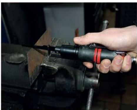
**SlimPOWER mini-pneumatic grinding machine for large pads**
