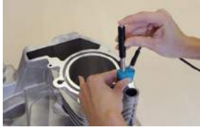
Figure 4: Leeb Testing Procedure
