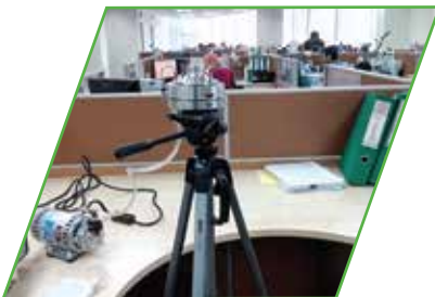
Indoor Air Quality Monitoring (IAQ)
