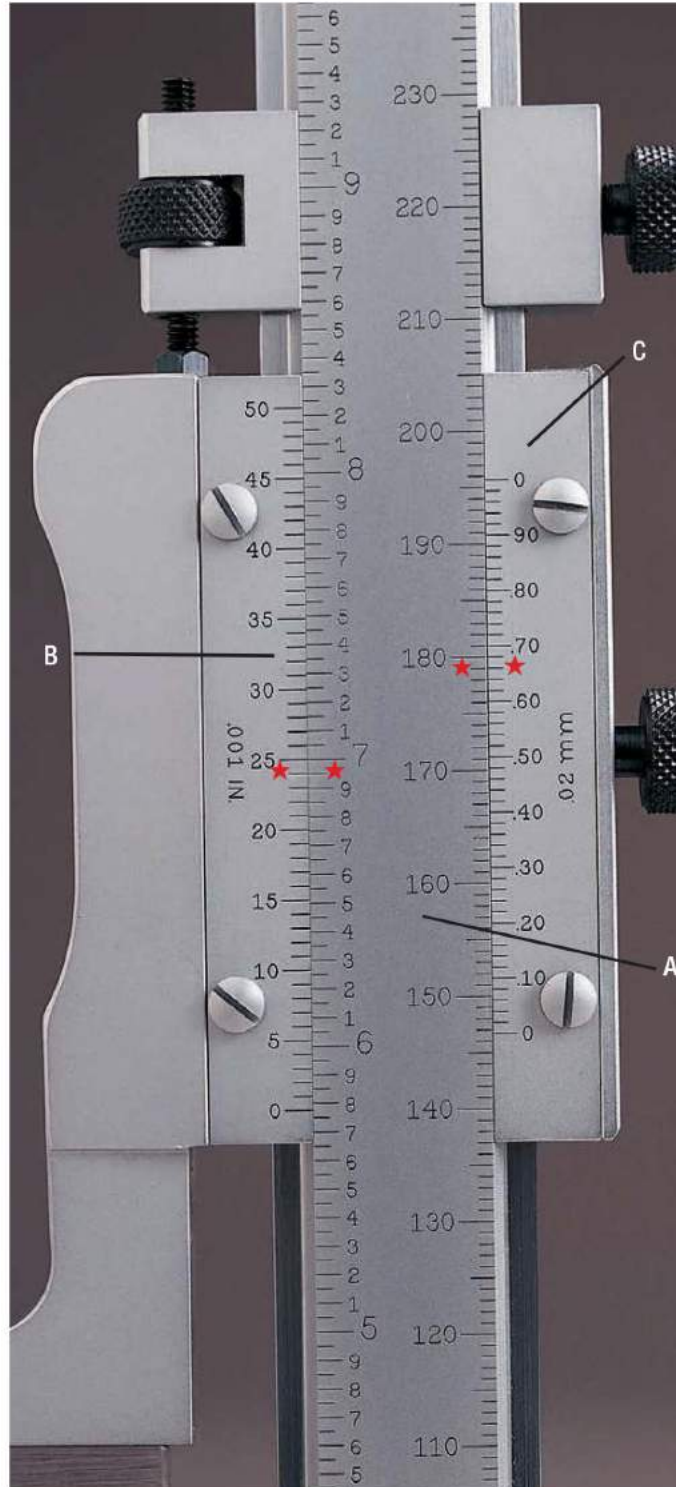
Open-face long Vernier with 50 widely spaced graduations for easy reading. Flush-fitting Vernier and master bar eliminates parallax.
