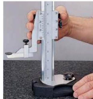
Quick-adjusting screw release allows rapid slide movement to desired area, then precisely position with the fine adjustment knob
