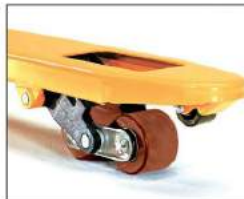
Tandem rollers Two adjustable rollers housed in each fork. Advantageous for uneven surfaces and when going over edges and bumps. Locating wheels at fork tips.
