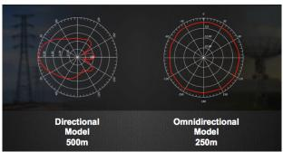
Built-in Directional and Omnidirectional Antennas of AP630
