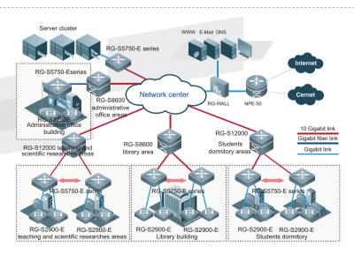
Typical 10 Gigabit Ethernet Backbone Campus Network Topology Diagram
