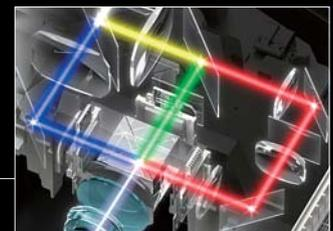
It is separated into red, green and blue through dichroic mirrors. After this, each of the three colours pass through LCD panels, producing three individual images. Lastly, these three images are transmitted through a prism and combined into the final full-colour image.
