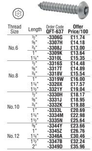
A2 Stainless Steel - Button Head Pin Hex security screws with internal pin within the socket prevents the use of standard hex keys. Suitable for medium torque applications.
