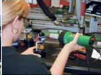
Shrinking a solder sleeve with TRIAC PID.
