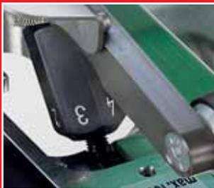
Adjustment of welding force for different materials
